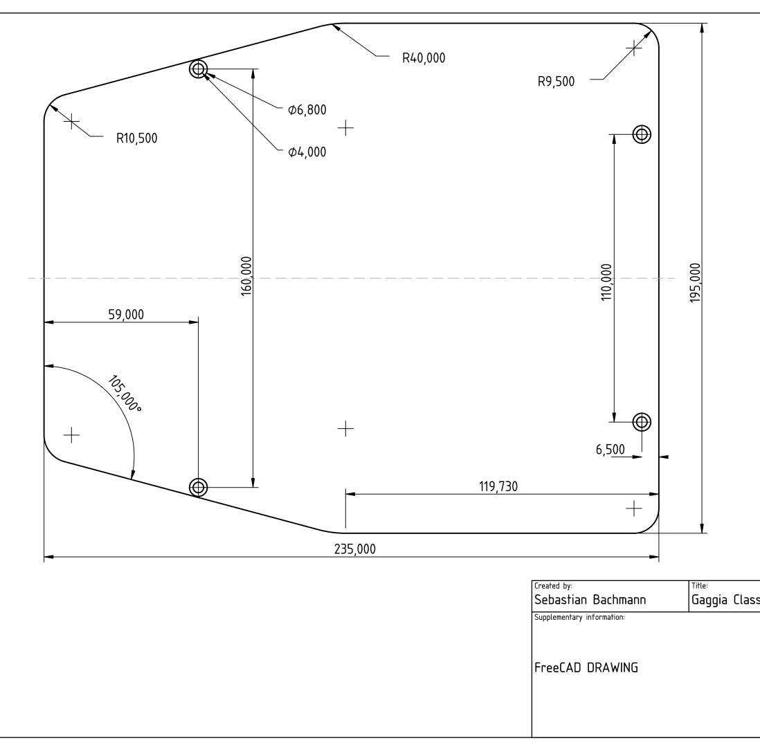
The Gaggia Classic allows for a 10mm plate, to be flush with the housing.
